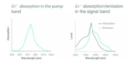
The design of our Host dopant system is currently as follows: Yttrium Silicide as our Host, and Erbium as our dopant. Above you can see the absorption spectrum of Erbium. The Bandgap of Yttrium Silicide is 4.77eV. You can see the Crystal structure of the host below. The Large bandgap of our host and the fact that it's spacing is large enough to support Er doping means that it is an ideal candidate for our Qubit.
